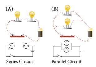
Figure 4.11 Series and parallel connections
