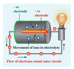
Figure 4.4 Electric current
