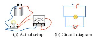
Figure 4.8 Connection of voltmeter in a circuit
