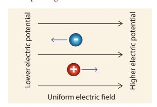
**Figure 4.3** Electric potential and Electric field
