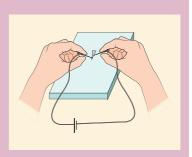
board. Connect a thin pin to two lengths of wire. Connect the wires to the terminals of electric cell, may be of 9V. Press one pin onto the pointed tip and other pin at a point about one or two mm away. Can you see that the tip of aluminium foil starts melting?
