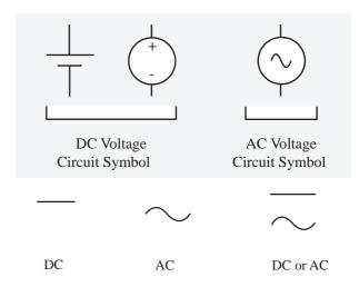
Figure 4.15 The symbol used in ac and dc circuit diagrams
