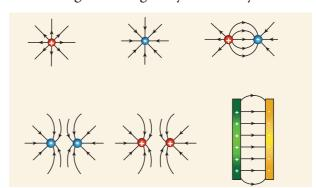
Figure 4.2 Electric lines of force
