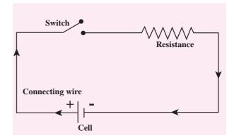
Figure 4.10 Typical electric circuit
