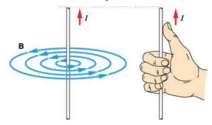
**Figure 4.12** Direction of current and magnetic field
