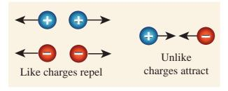
Figure 4.1 Electrostatic forces
